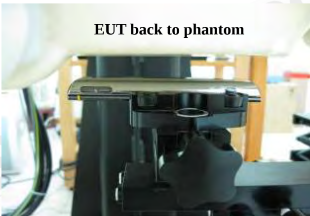
Fig.12 Body worn- EUT back to flat phantom and distance between flat phantom and mobile phone is 1.5 cm
