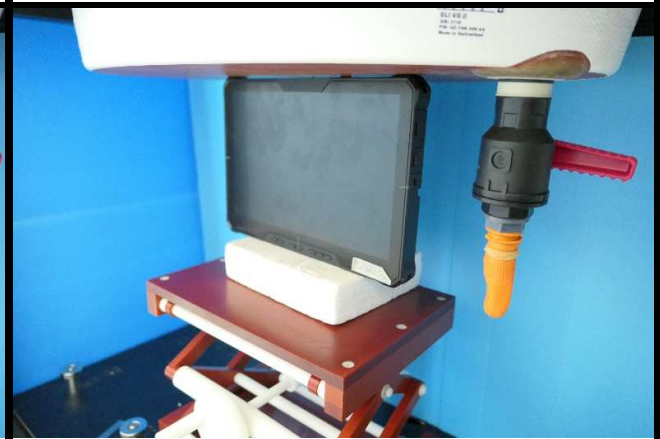
Top Side of EUT Tested at 0 mm
