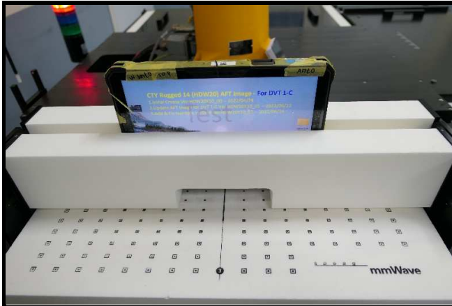
Rear Face of EUT Tested at 0 mm
