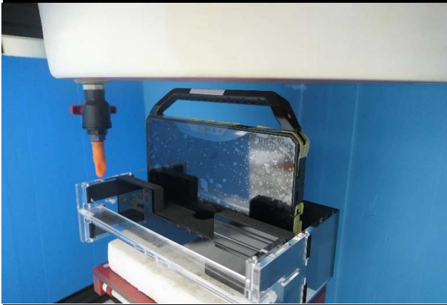
Top Side of Tablet Mode Tested at 10 mm_Handheld
