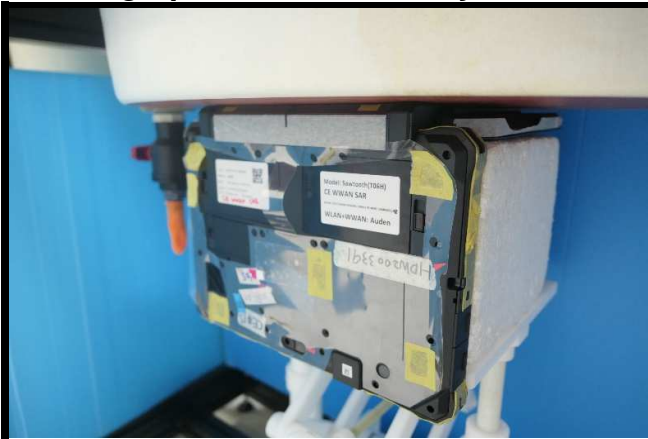
Bottom of EUT Tested at 0 mm
