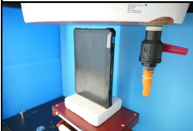
Right Side of EUT Tested at 15 mm
