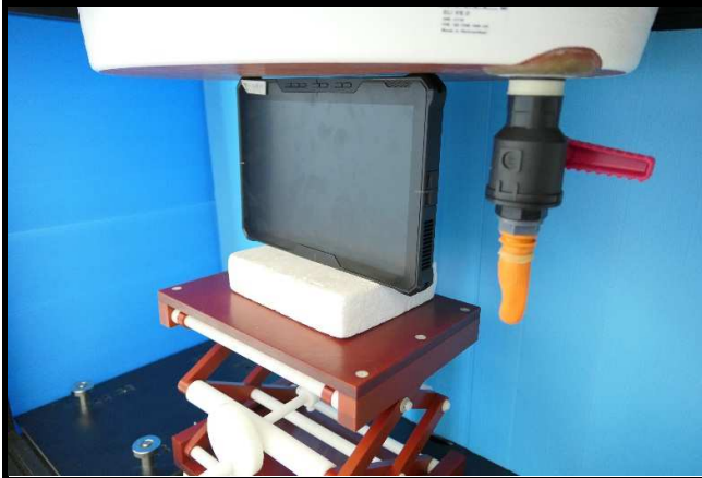
Bottom Side of EUT Tested at 0 mm
