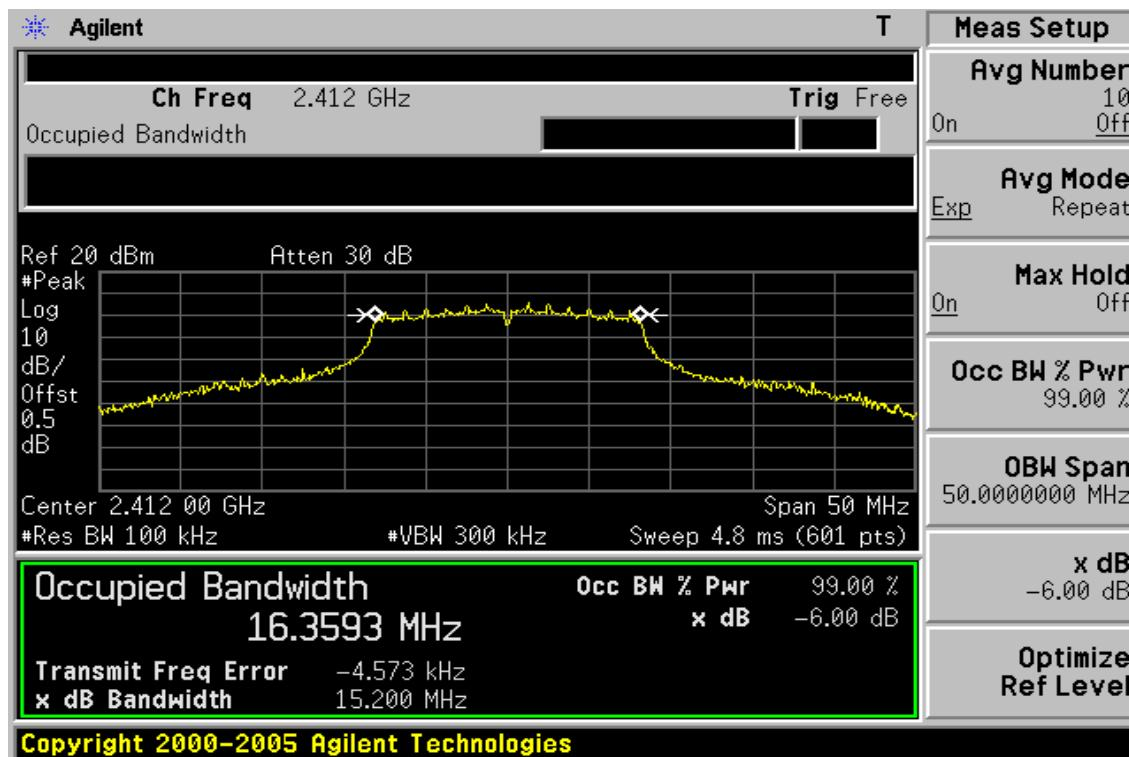
**6dB Band Width Test Data CH-Mid**
