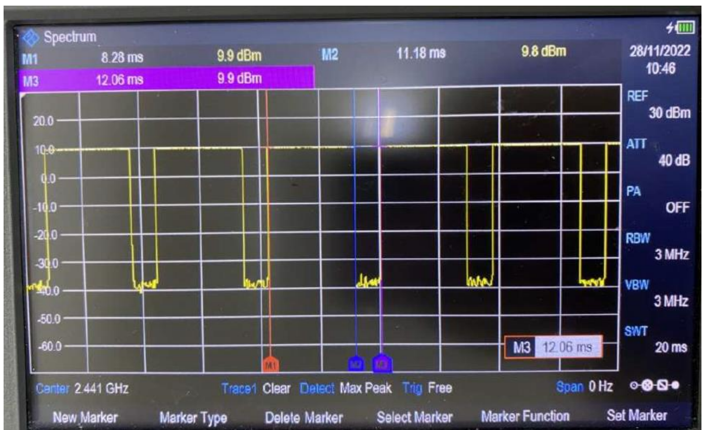
Time-domain plot for Bluetooth transmission signal
