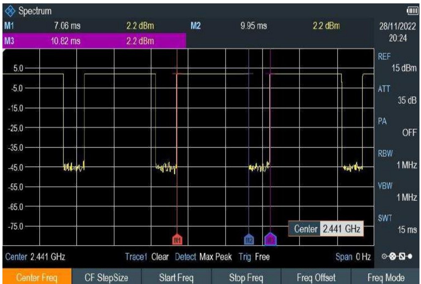
Time-domain plot for Bluetooth transmission signal
