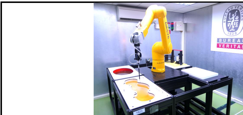
Fig-3.2 SPEAG DASY6 System
