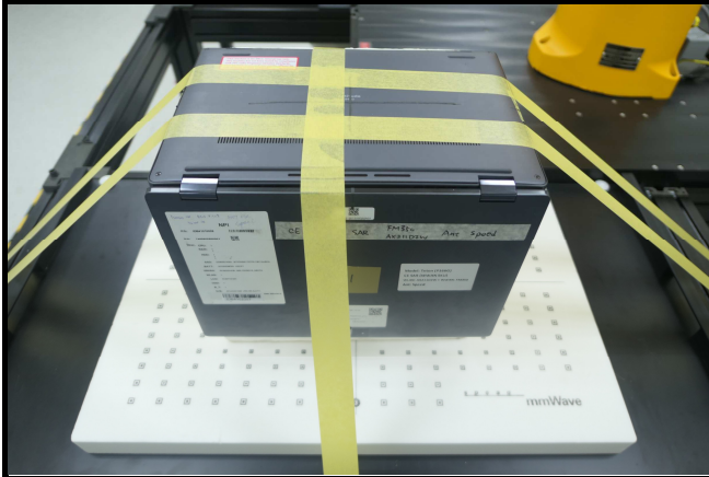
Bottom of EUT Tested at 0 mm
