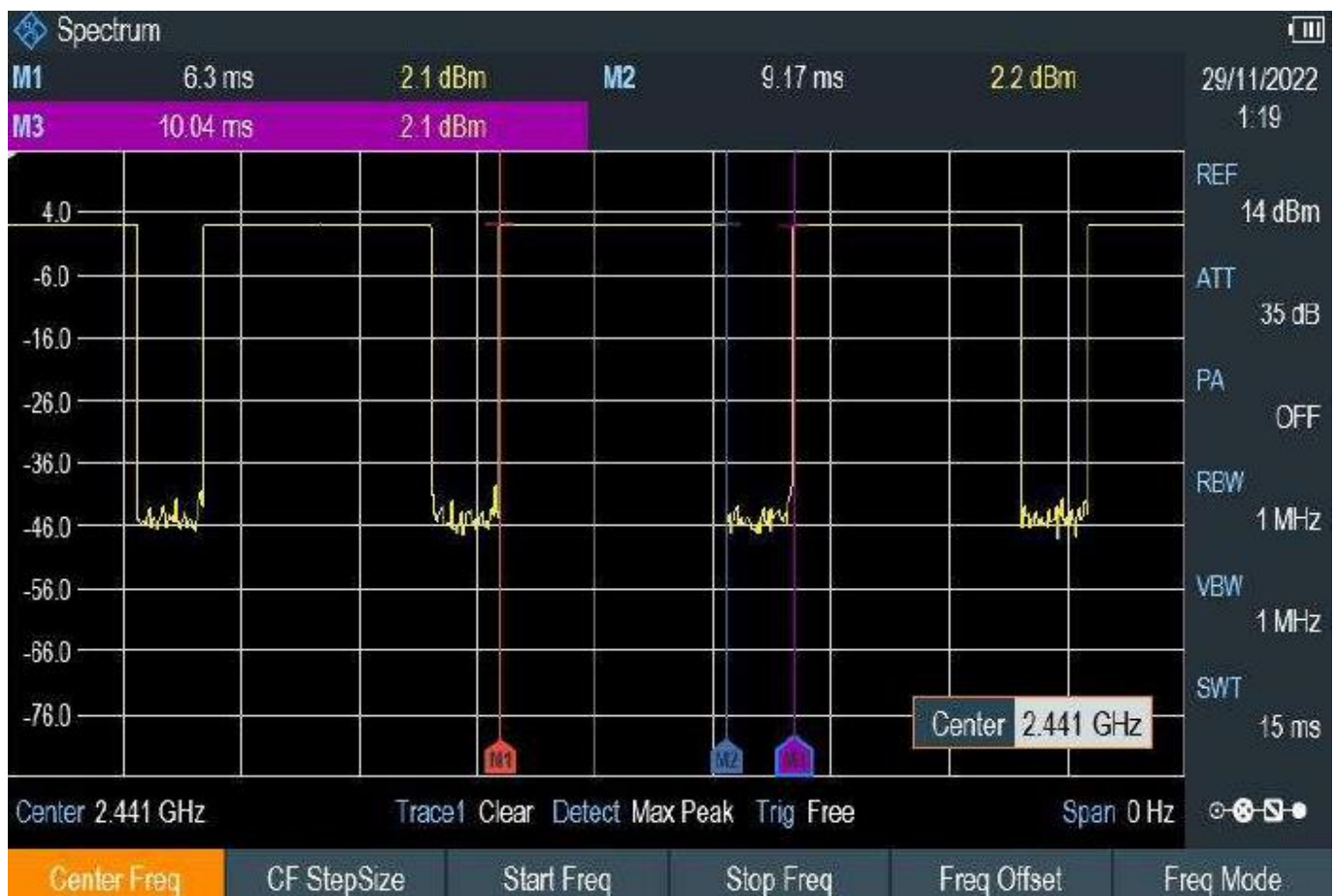
Time-domain plot for Bluetooth transmission signal
