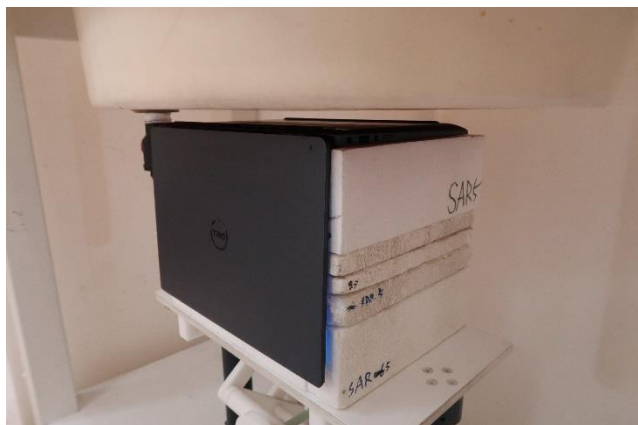
Bottom of Laptop at 18 mm
