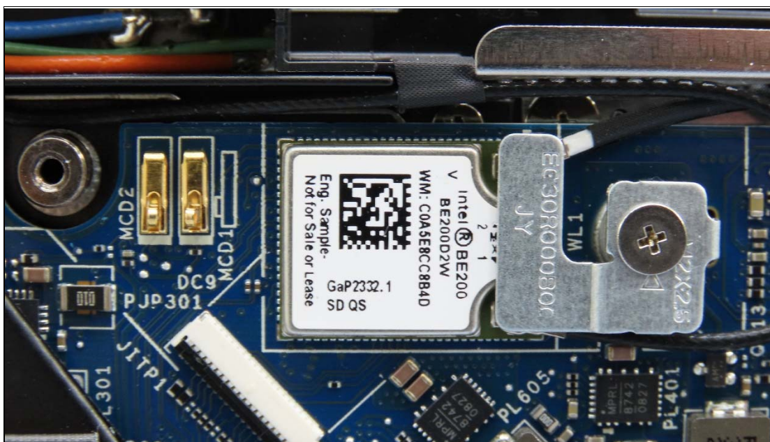
BT + WiFi module (Brand: Intel® BE200D2W, Model: BE200D2W)
