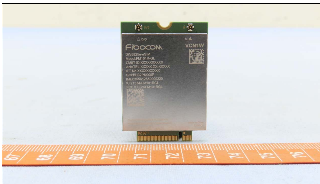
WWAN module (Brand: Fibocom, Model: FM101R-GL)
