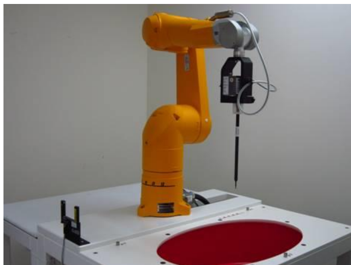
Fig.1 Photograph of the SAR measurement system
