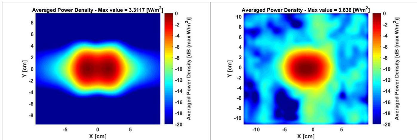
The plots below show the comparison between the numerical modeling and the system check results in terms of normalized E-field distribution and the 1D variation along the two axis of the maximum.
