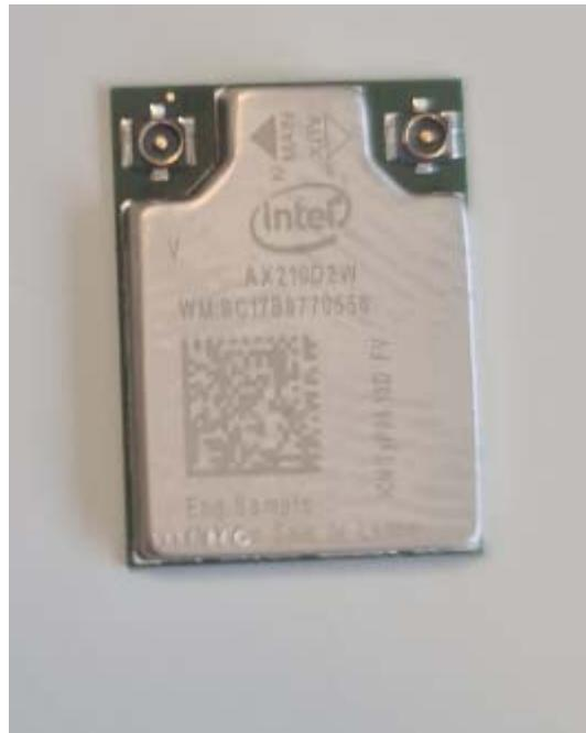
Note: Due to the small device size 12mm x 16mm it is too small to imprint the FCCID and IC ID on the module. The font size required would need to be < size 4 font and is considered to require magnification for legibility. The ID's will be placed in the Information Guide. External host labeling is still required once integrated into host.
