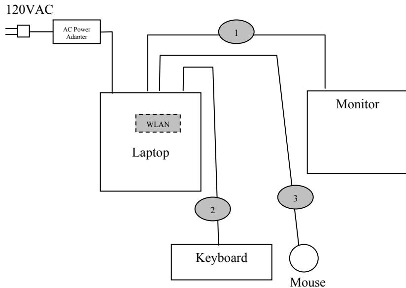
Cable 1: This is a 6-foot braid and foil shielded round cable connecting the host computer with the monitor. It has metallic DB-15 type connector at the computer end and is hardwired to the monitor. The cable is bundled to a length of one meter and the shield of the cable is grounded to the chassis of both devices via the connector shells.
