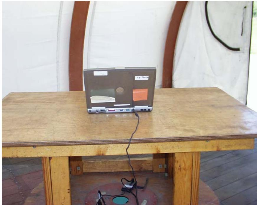
**POWERLINE CONDUCTED EMISSIONS MEASUREMENT SETUP**
