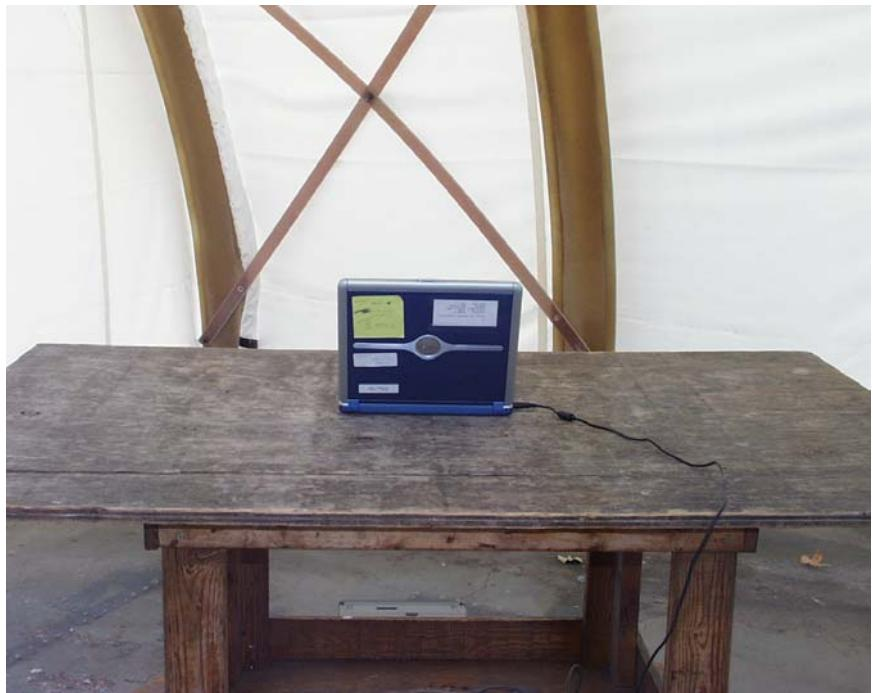
**POWERLINE CONDUCTED EMISSIONS MEASUREMENT SETUP**
