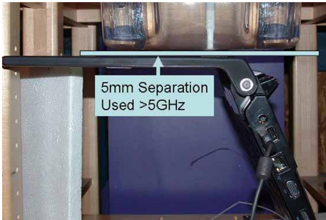
Position of the Laptop During 5mm Separation Testing
