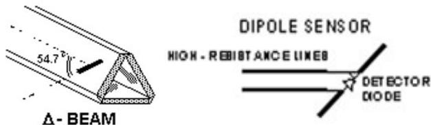
SAR is assessed with a calibrated probe which moves at a default height of 1.4mm from the centre of the diode, which is mounted to the sensor, to the phantom surface (in the Z Axis). The 1.4mm offset height has been selected so as to minimize any resultant boundary effect due to the probe being in close proximity to the phantom surface.
