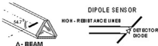
SAR is assessed with a calibrated probe which moves at a default height of 4mm from the centre of the diode, which is mounted to the sensor, to the phantom surface (in the Z Axis). The 4mm offset height has been selected so as to minimize any resultant boundary effect due to the probe being in close proximity to the phantom surface.
