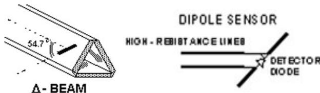
SAR is assessed with a calibrated probe which moves at a default height of 5mm from the centre of the diode, which is mounted to the sensor, to the phantom surface (in the Z Axis). The 5mm offset height has been selected so as to minimize any resultant boundary effect due to the probe being in close proximity to the phantom surface.
