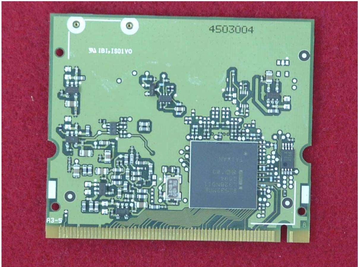
***Bottom View of the WLAN Transmitter
