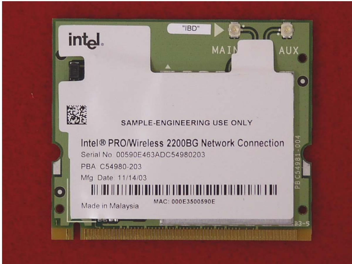
*Top View of the WLAN Transmitter
