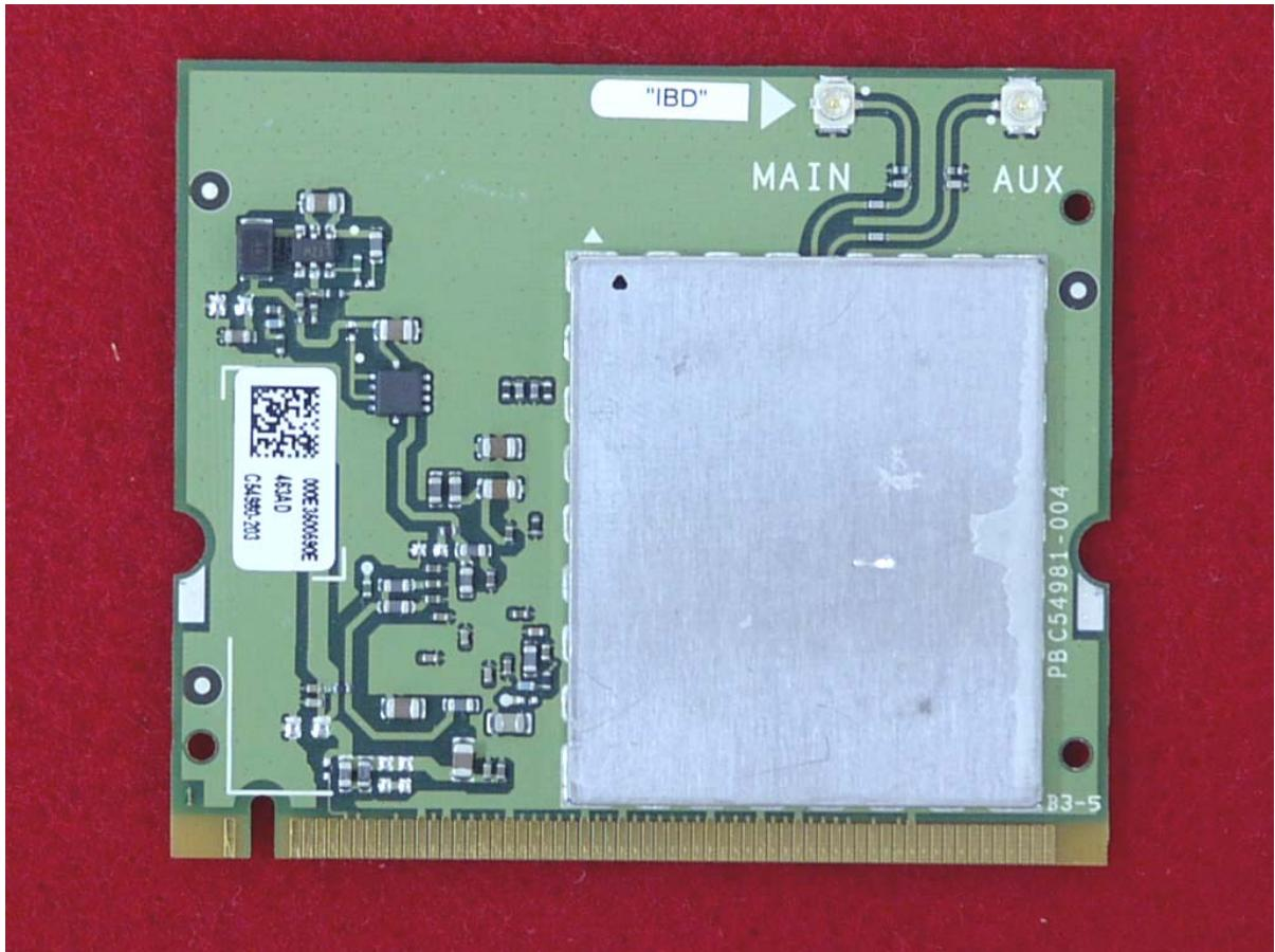
*Top View of the WLAN Transmitter
