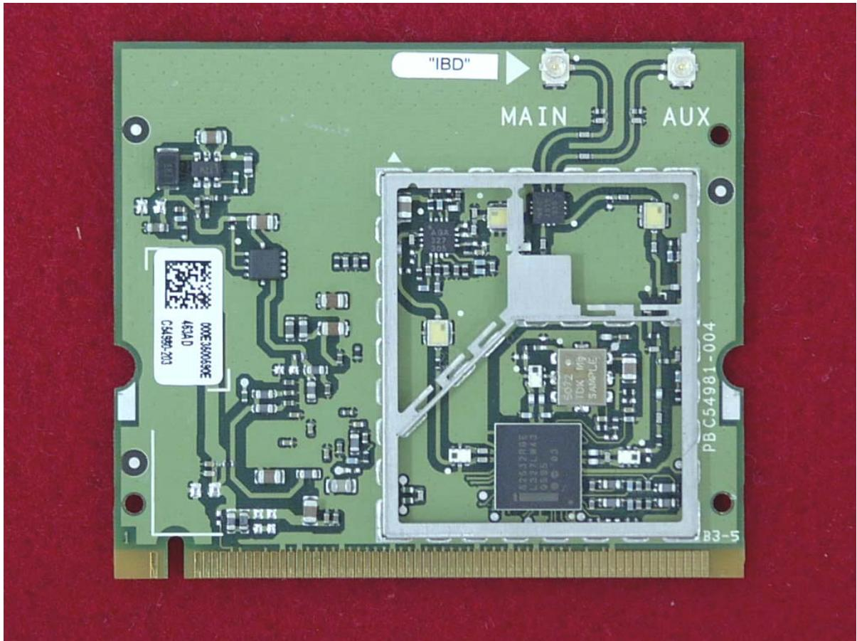
*Top View of the WLAN Transmitter
