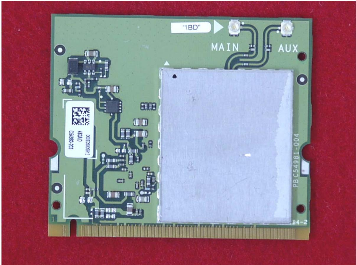
*Top View of the WLAN Transmitter
