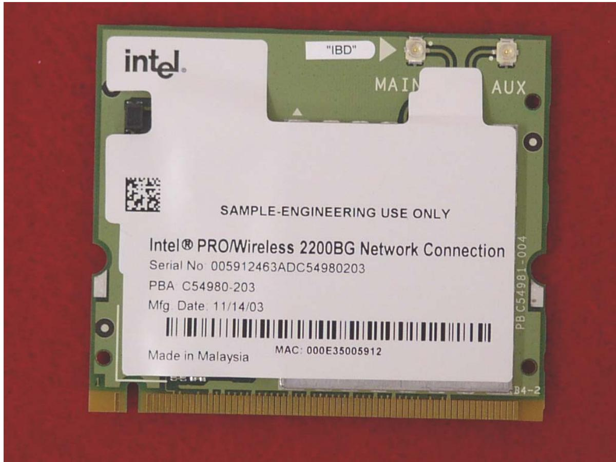
*Top View of the WLAN Transmitter
