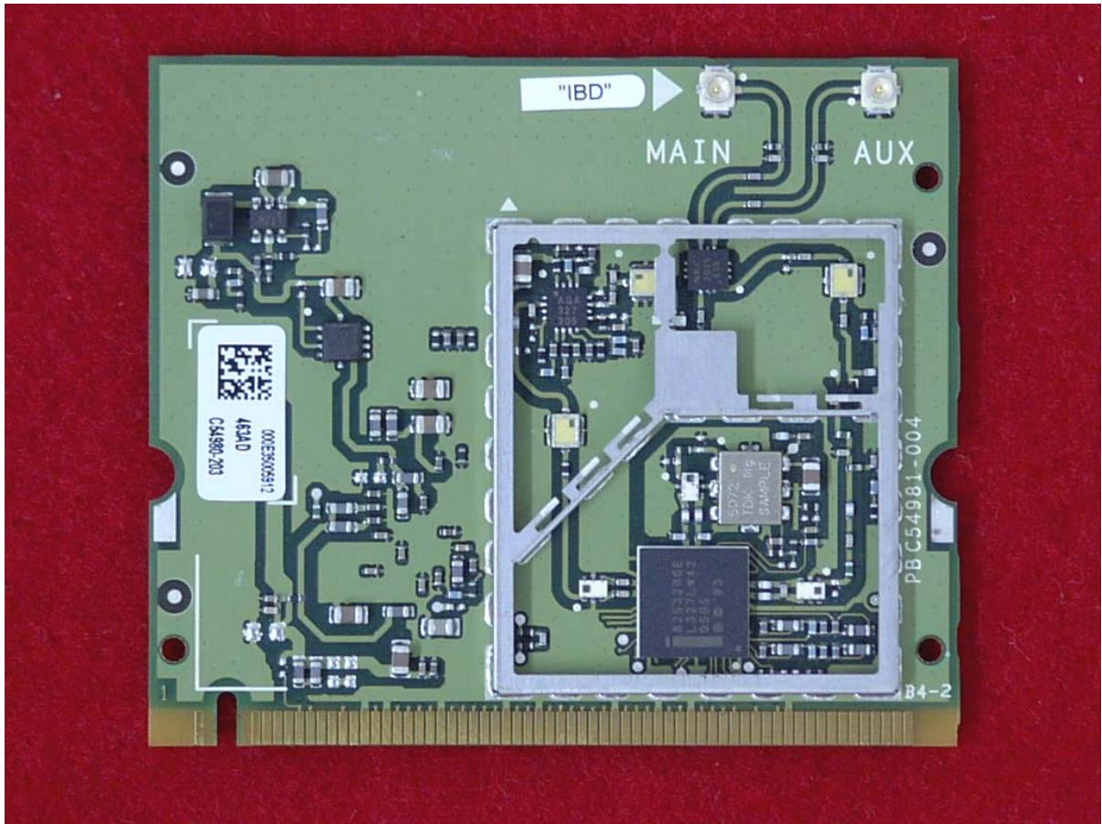
*Top View of the WLAN Transmitter
