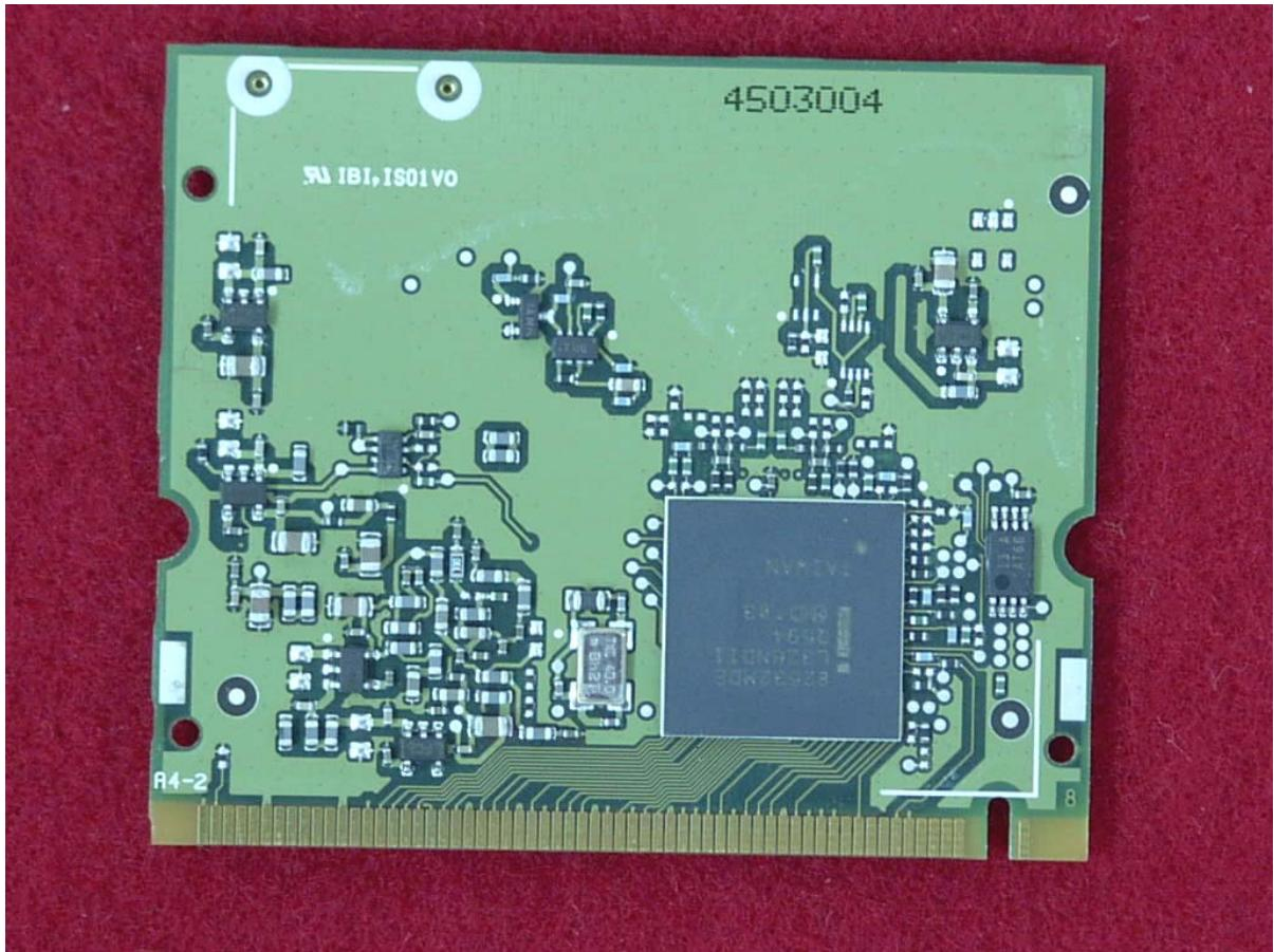
*Bottom View of the WLAN Transmitter
