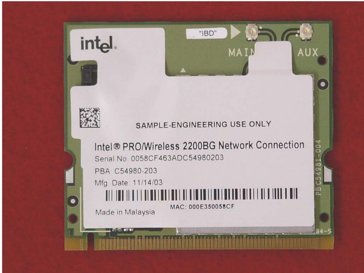
*Top View of the WLAN Transmitter
