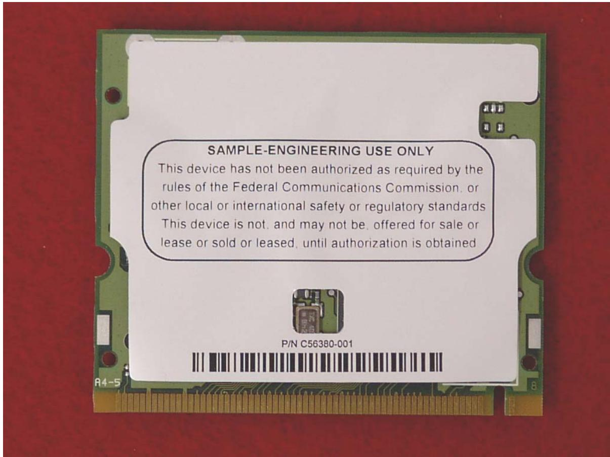
***Bottom View of the WLAN Transmitter
