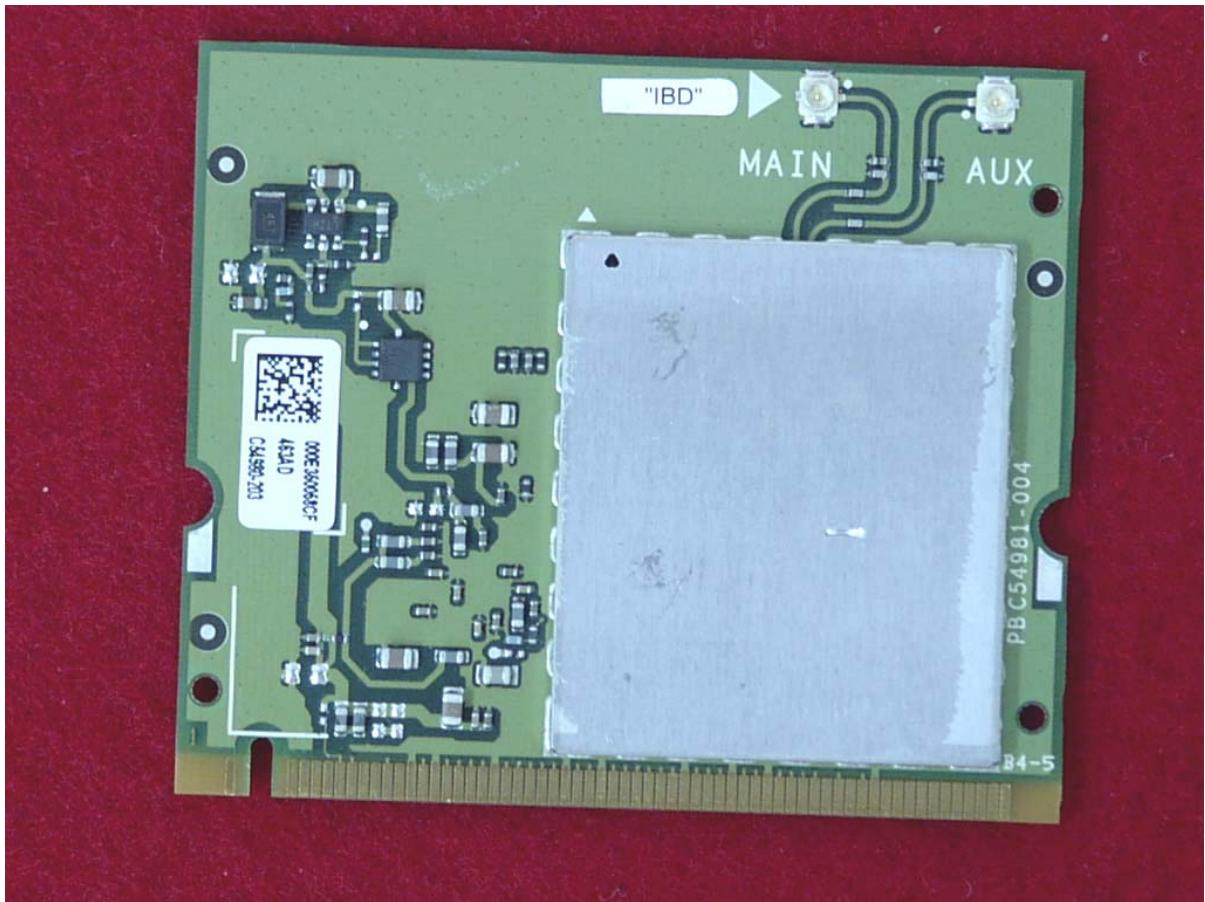
*Top View of the WLAN Transmitter
