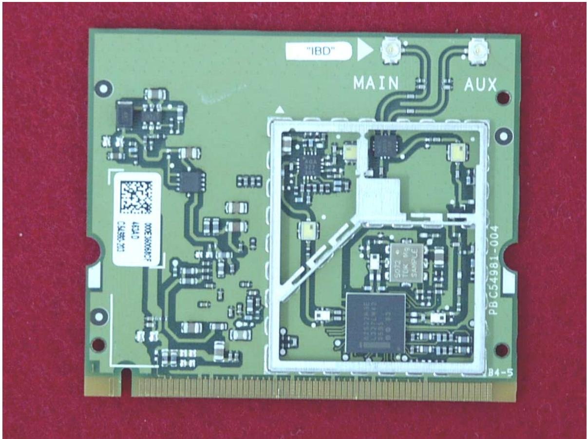
*Top View of the WLAN Transmitter
