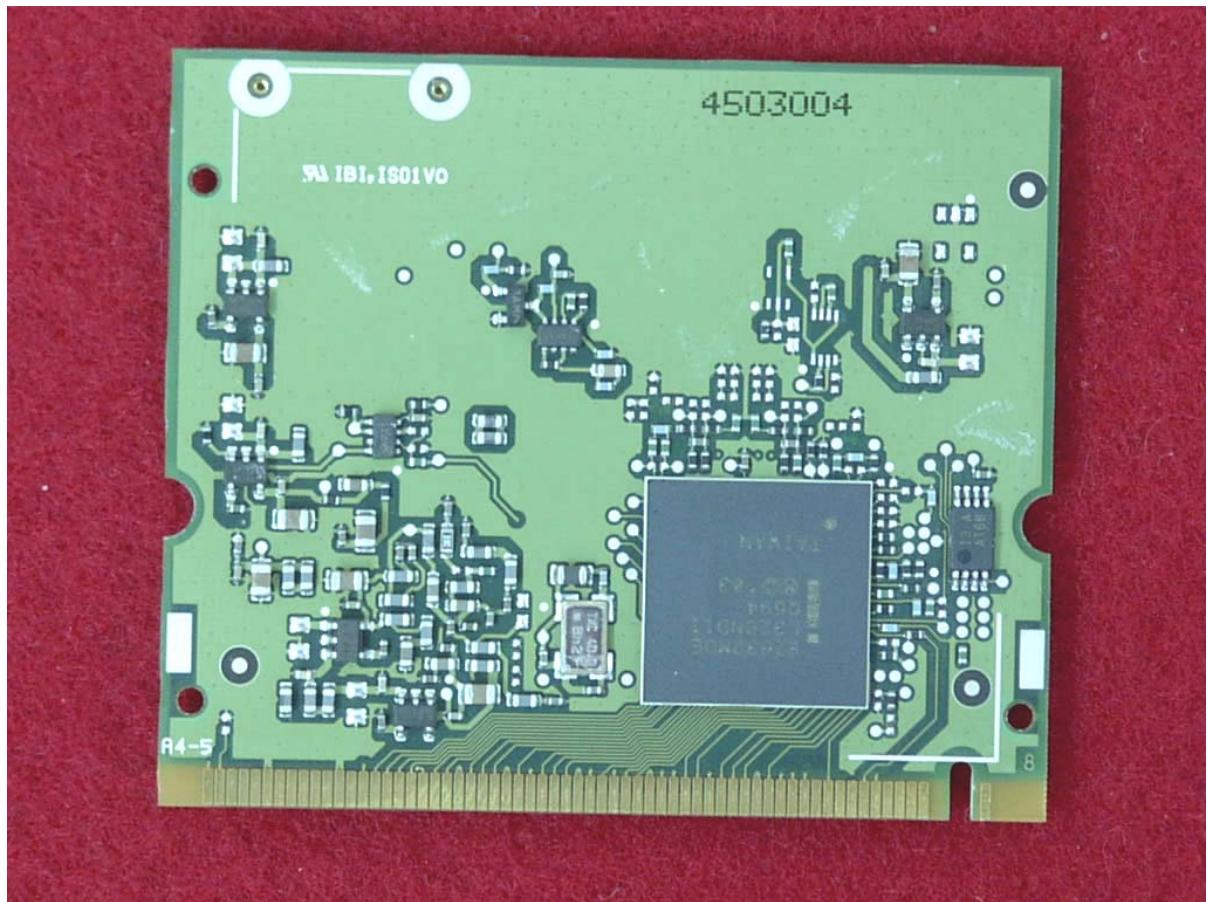
***Bottom View of the WLAN Transmitter
