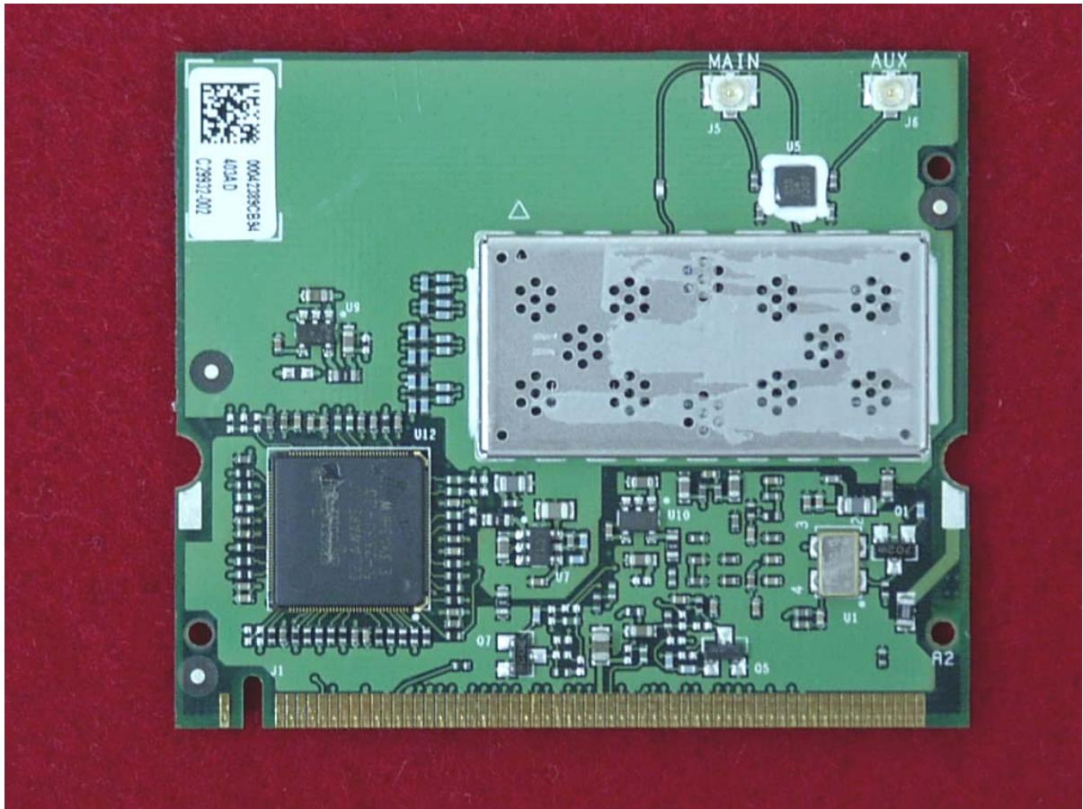
*Top View of the WLAN Transmitter
