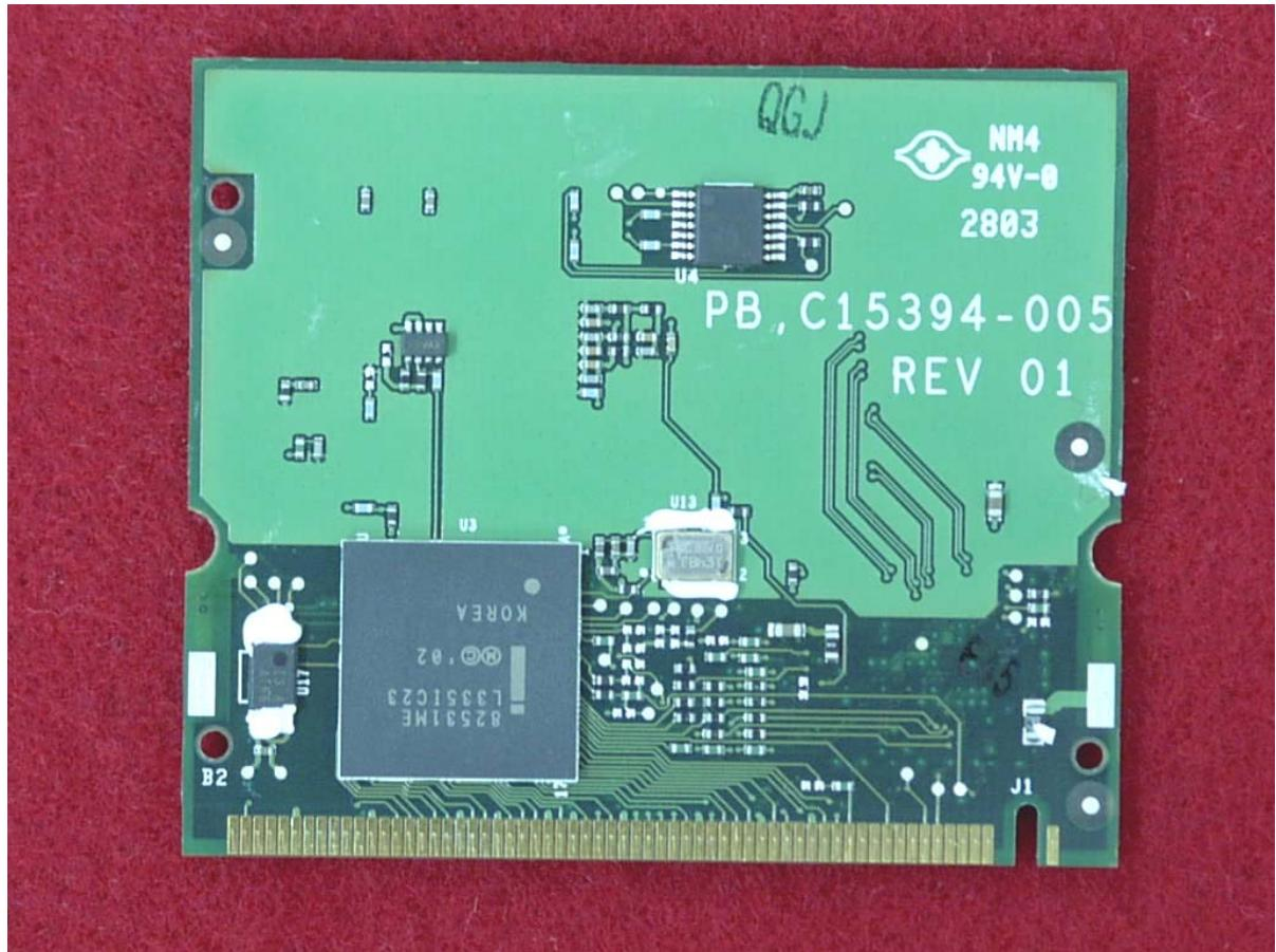
*Bottom View of the WLAN Transmitter
