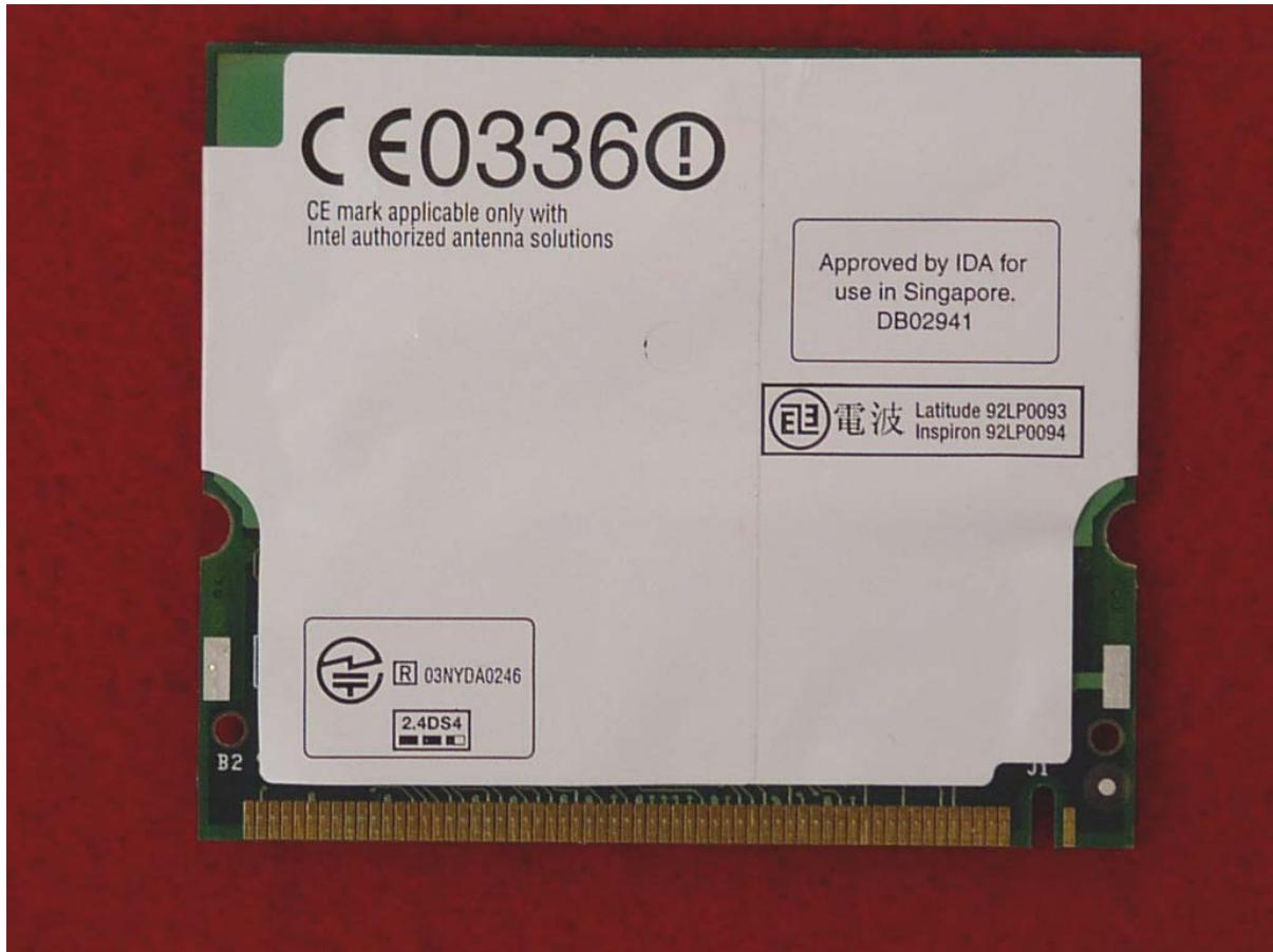
***Bottom View of the WLAN Transmitter
