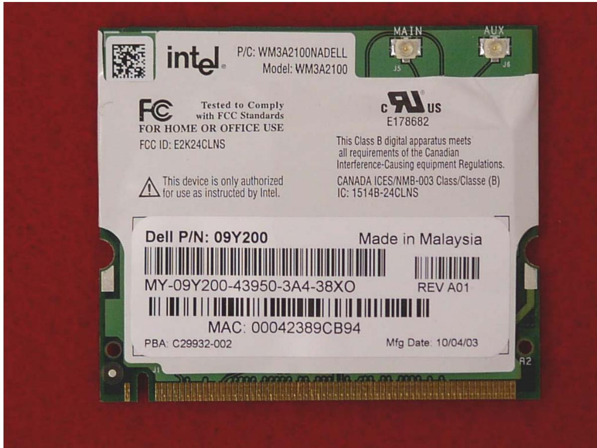
*Top View of the WLAN Transmitter
