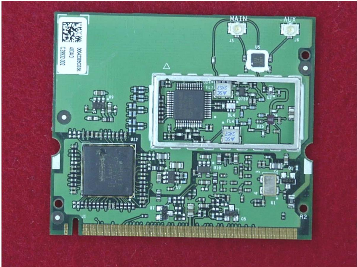
*Top View of the WLAN Transmitter
