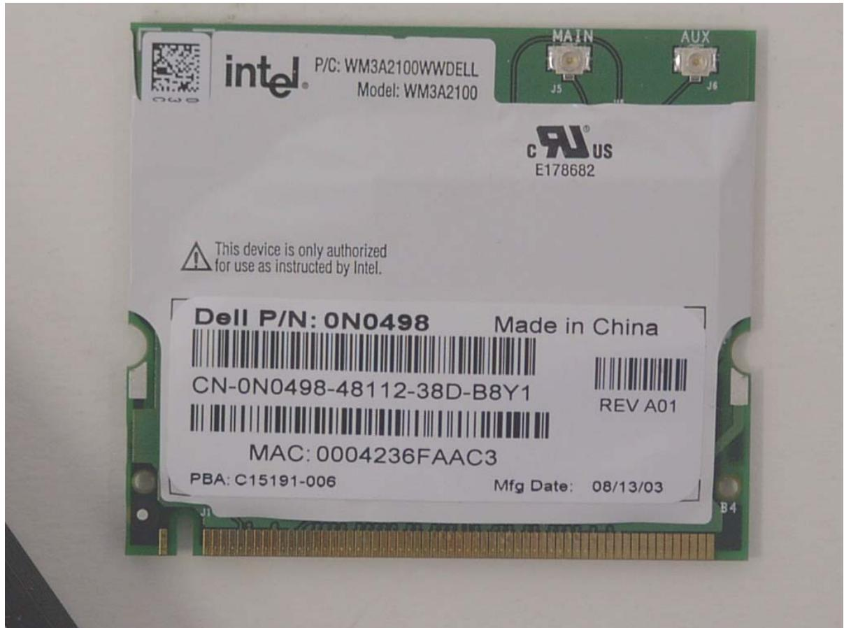
*Top View of the WLAN Transmitter
