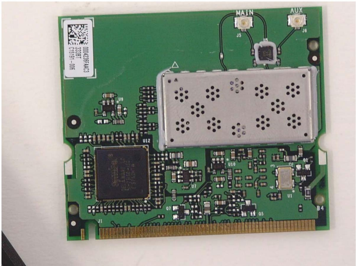
*Top View of the WLAN Transmitter
