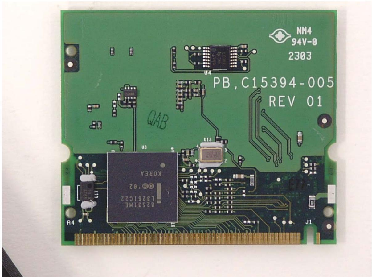
*Bottom View of the WLAN Transmitter
