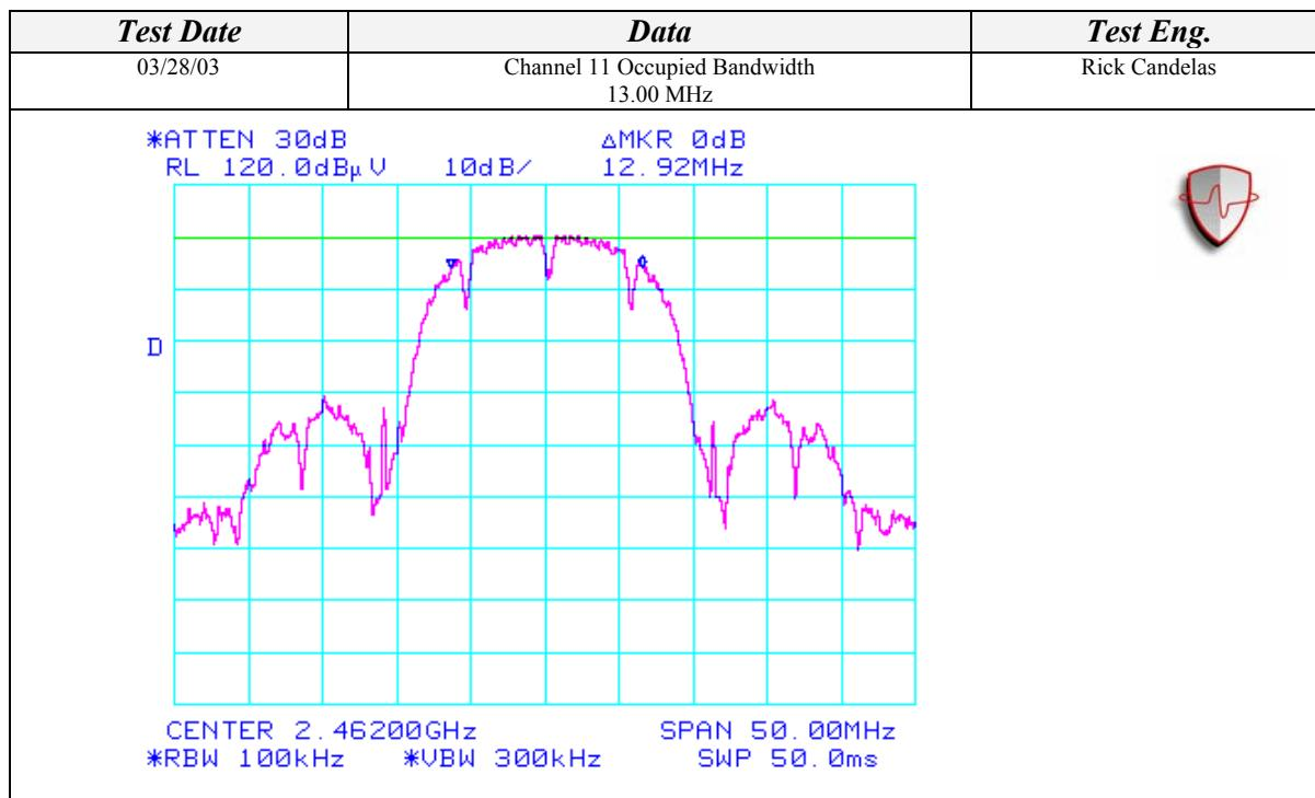
**SPECTRAL POWER DENSITY MEASUREMENT**
