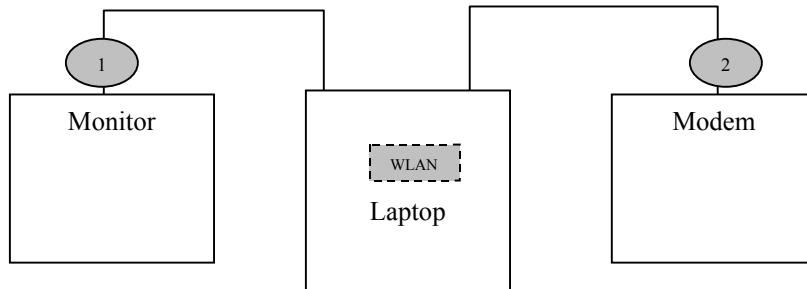
Cable 1: This is a 6-foot braid and foil shielded round cable connecting the host Dell Computer laptop computer with the NEC monitor. It has metallic DB-15 type connector at the computer end and is hardwired to the monitor. The cable is bundled to a length of one meter and the shield of the cable is grounded to the chassis of both devices via the connector shells.
