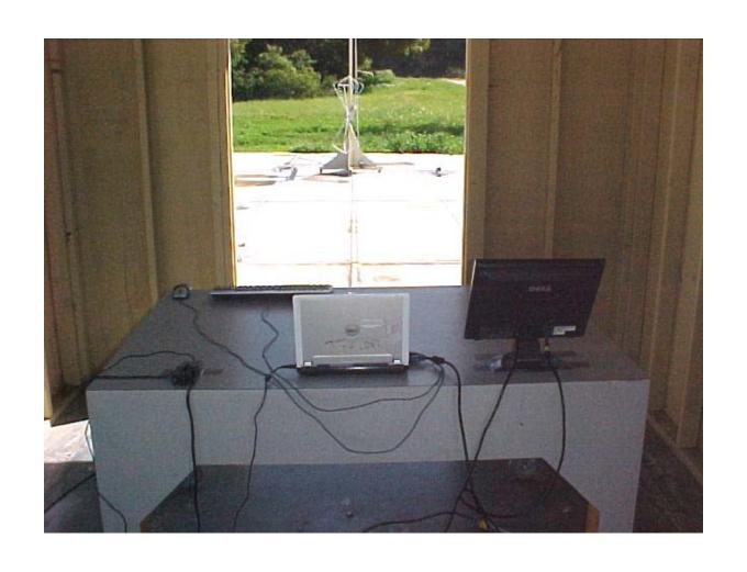
Radiated Emissions Measurement (30-1000 MHz) (Rear View) Setup
