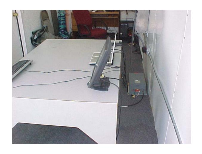
AC Conducted Emissions Measurement (Rear View) Setup
