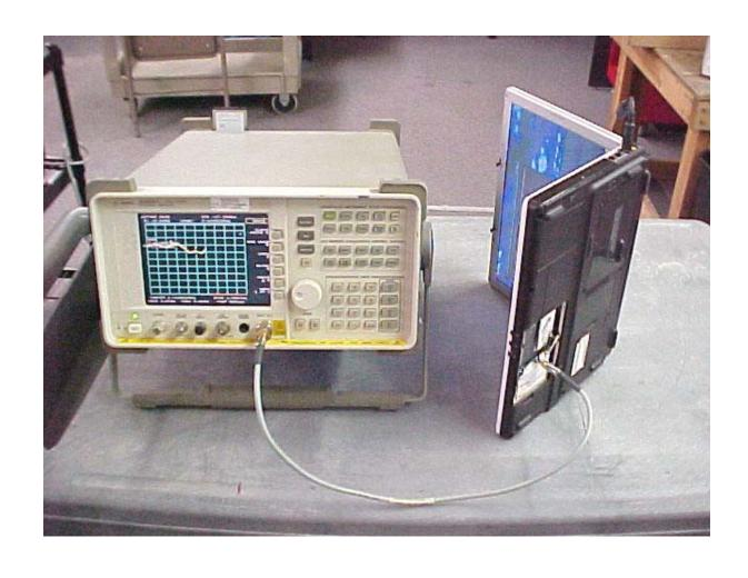
Conducted Emissions at Antenna Terminal Setup
