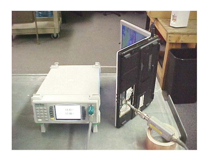
Maximum Peak Output Power Measurement Setup
