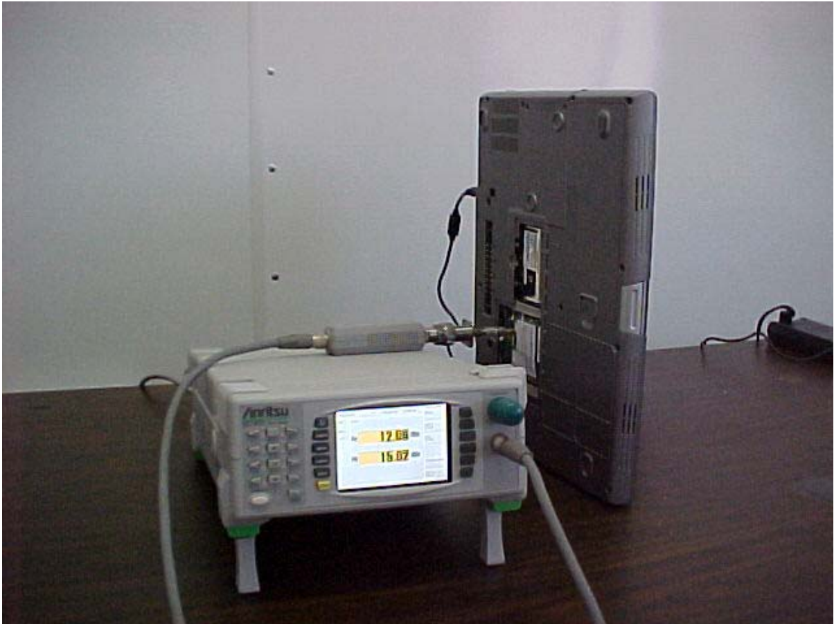
Maximum Peak Output Power Measurement Setup
