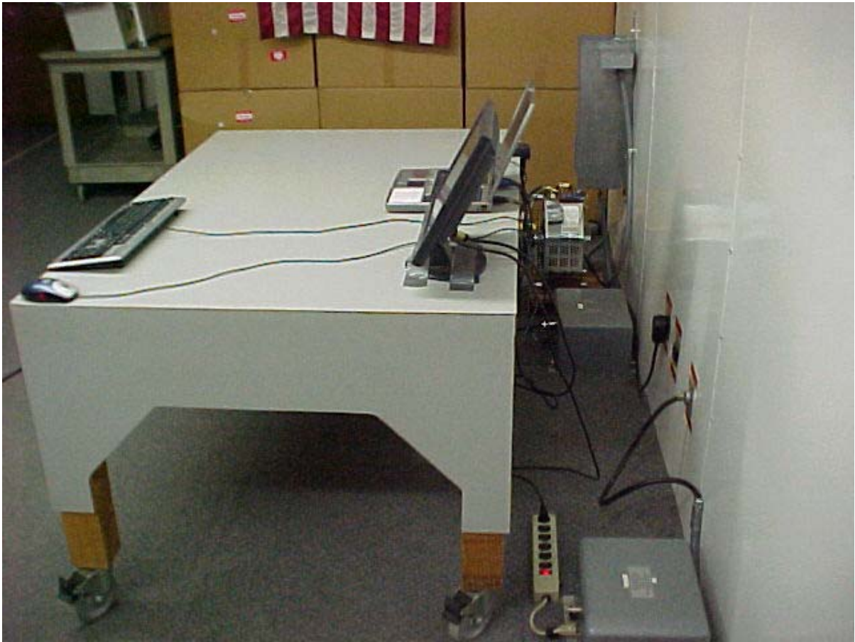
AC Conducted Emissions Measurement (Rear View) Setup
