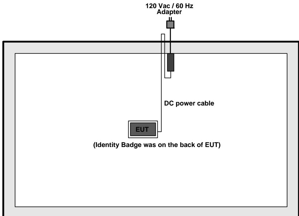
**Test Setup Diagram - Radiated 30MHz~1GHz Test**
