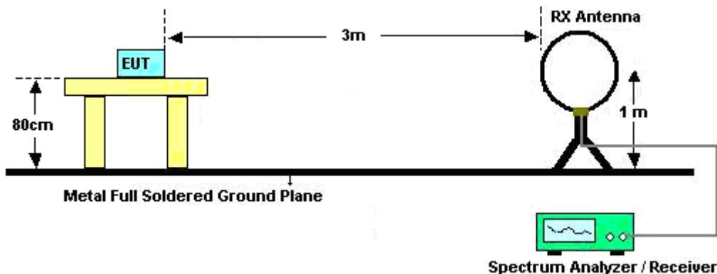
For radiated emissions from 30MHz to 1GHz
