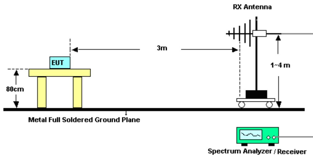
For radiated test from 1GHz to 18GHz
