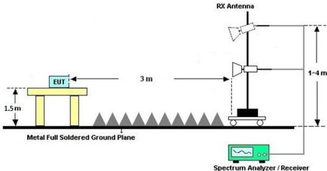
For radiated test above 18GHz
