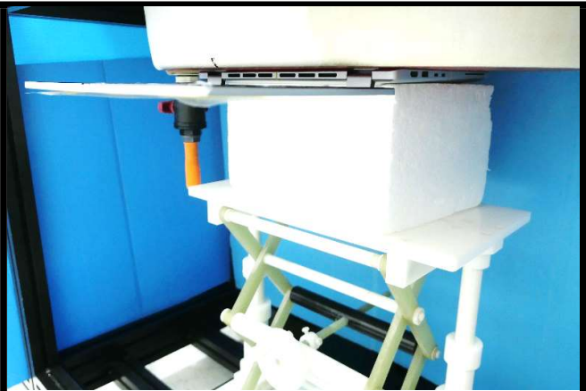
Keyboard Front Face of Laptop Tested at 0 mm
