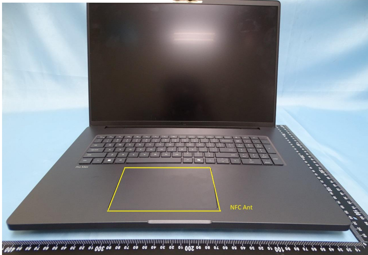
SPEED and Wistron NeWeb Corp. Antenna
