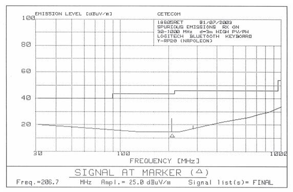
Resolution bandwidth = 100 kHz. Video bandwidih = 100 kHz.
