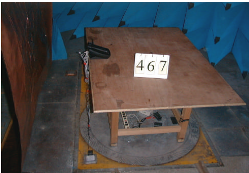
Fig. 2 Conducted Emissions Test Configuration (Operating only)
