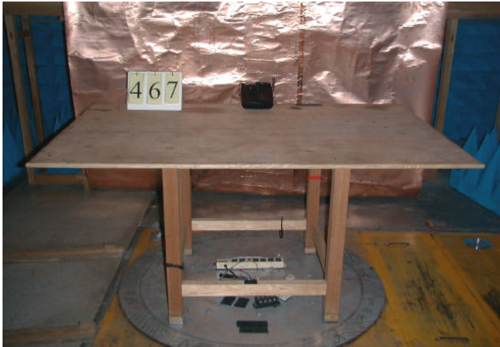
Fig. 1 Conducted Emissions Test Configuration (Operating only)
