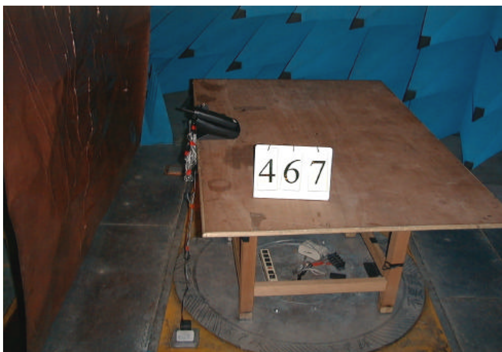
Fig. 2 Conducted Emissions Test Configuration (Charging only)
