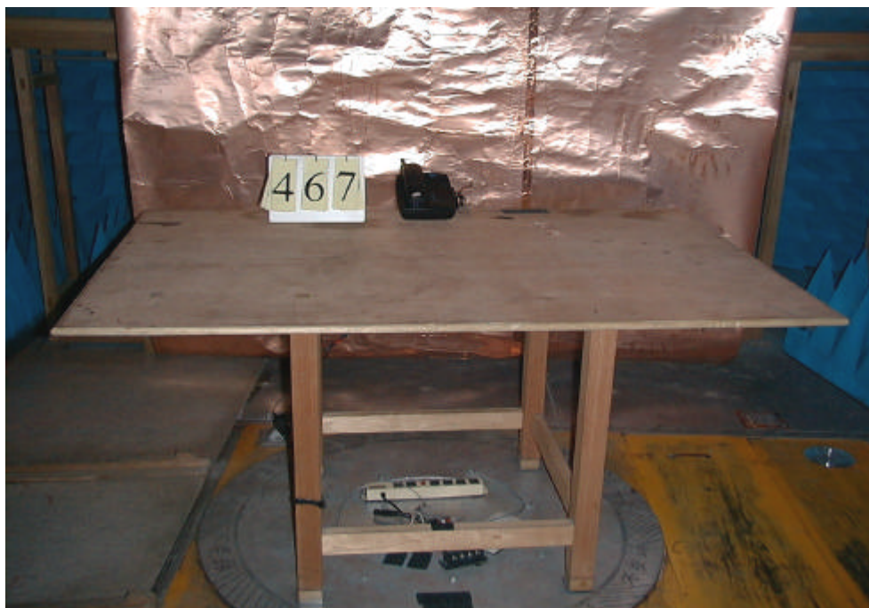
Fig. 1 Conducted Emissions Test Configuration (Charging only)
