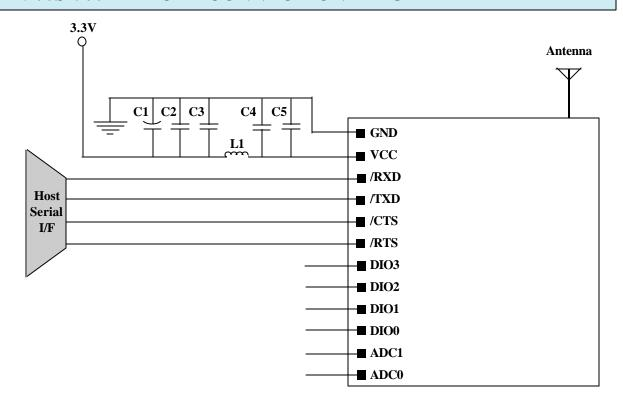
Parts List for XE900S-500 Typical Connection Diagram
