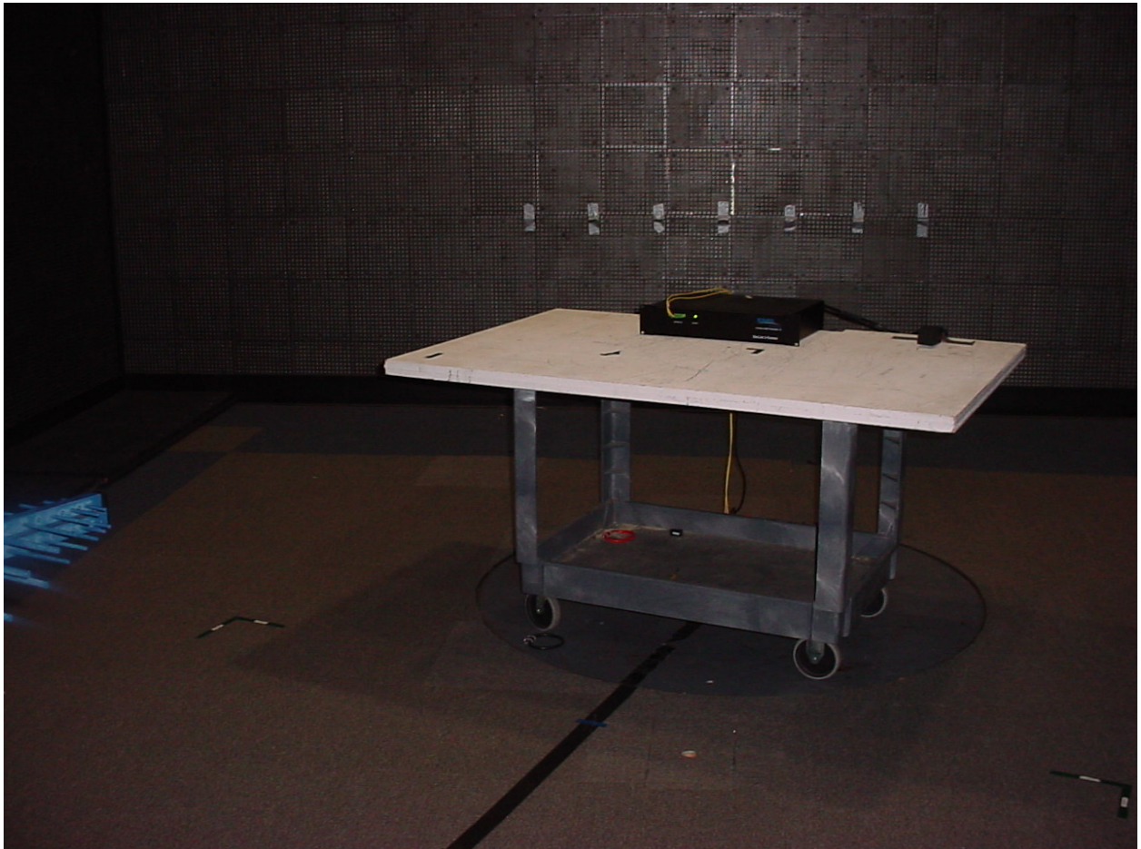
Figure 4: Test Setup – Radiated Emissions - Unintentional
