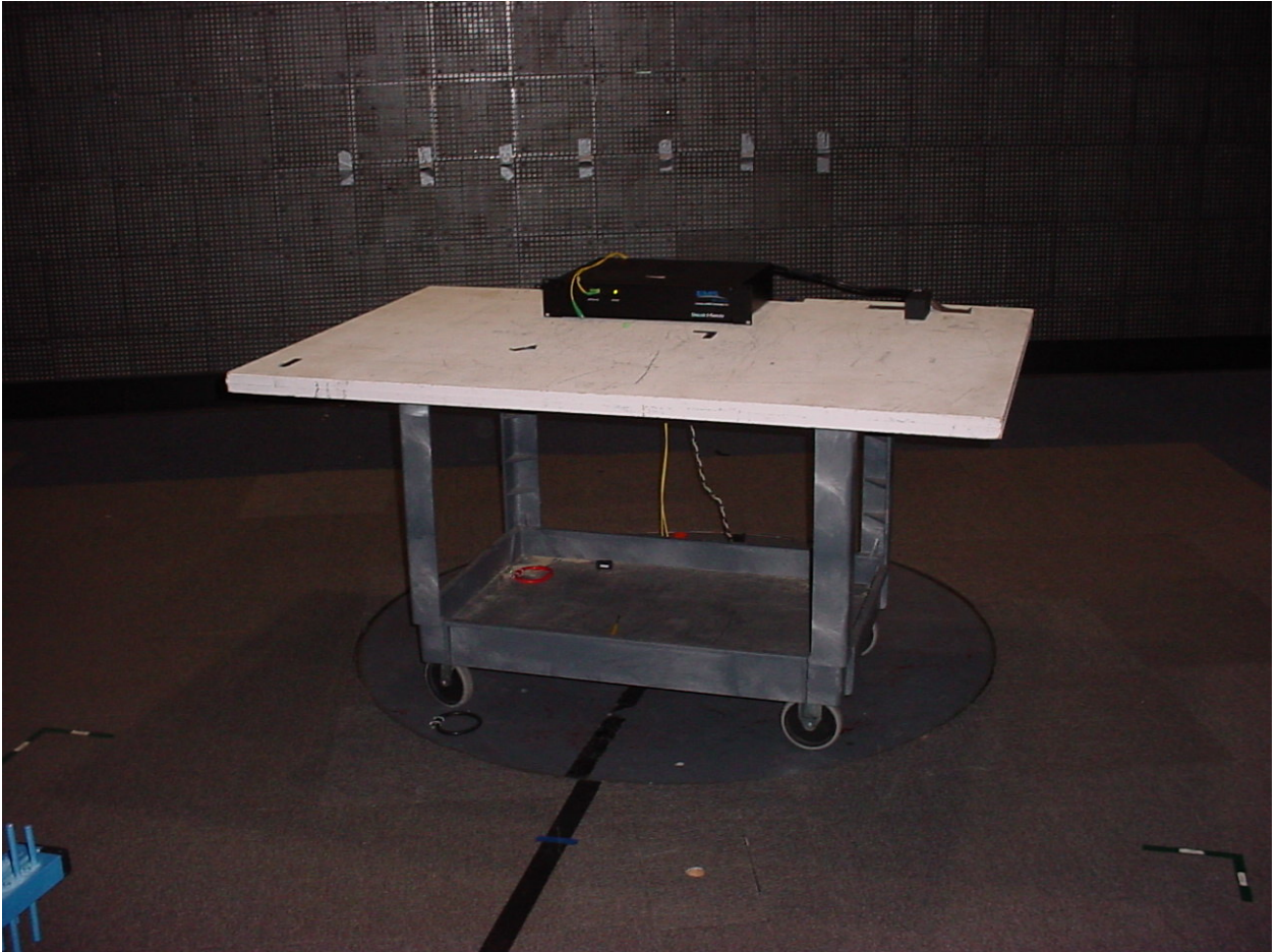
Figure 4: Test Setup – Radiated Emissions - Unintentional
