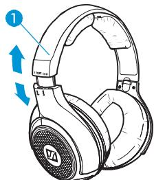
For good sound quality and best possible comfort, the headband has to be adjusted to properly fit your head. To do so, adjust the headband (1) via its snap-in locking mechanism:
