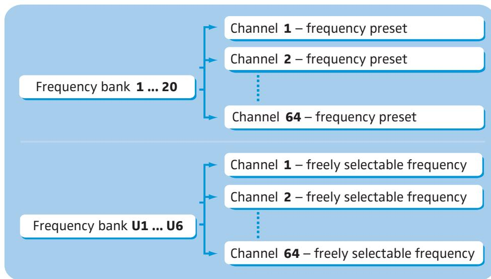
Each of the channels in the frequency banks “1” to “20” has been factory-preset to a fixed frequency (frequency preset). The factory-preset frequencies within one frequency bank are intermodulation-free. These frequencies cannot be changed.
