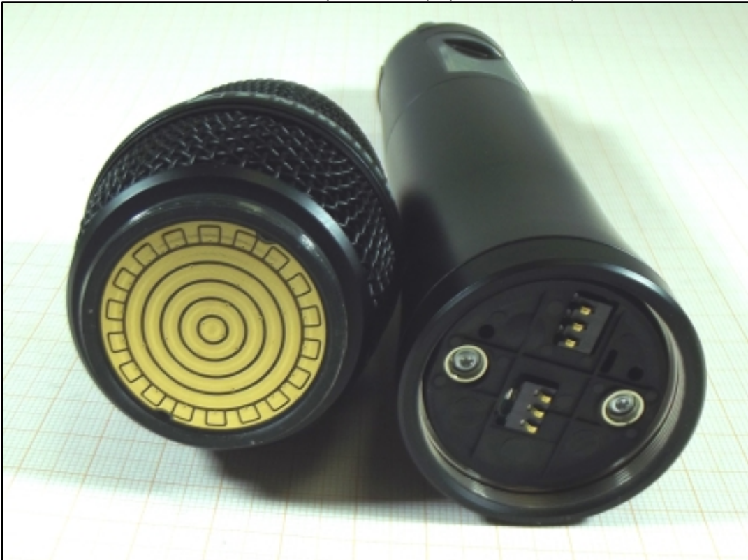
Photo 4: DUT - Top side view (capsule removed)
