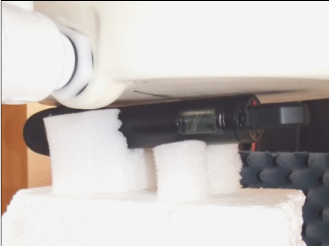
Photo 8: Test position - Bottom side with 0mm distance
