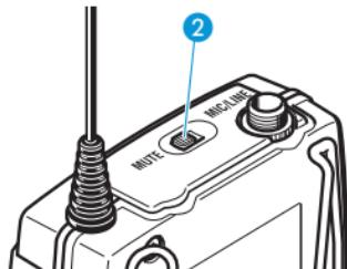
The **MUTE** switch 2 allows you to mute the audio signal or to deactivate the RF signal. Via the “**Mute Mode**” menu item, you can set the desired function of the **MUTE** switch 2.
