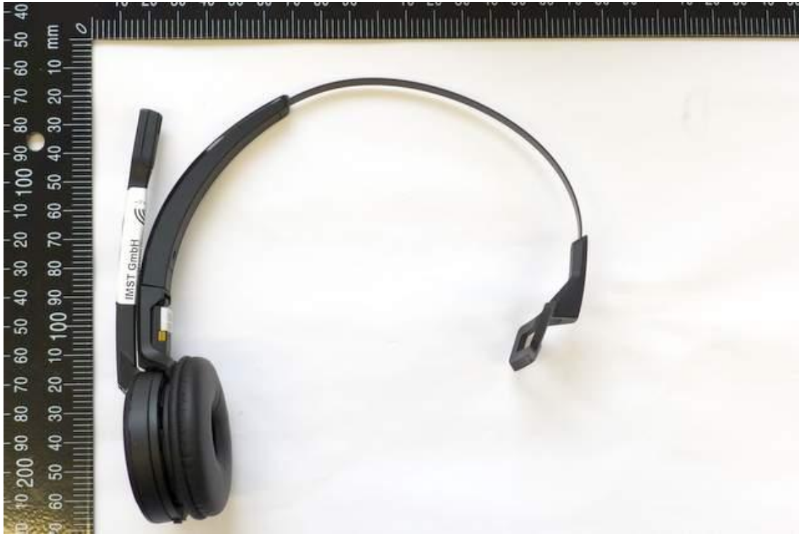
Pic. 3: View of the device under test with attached metal head band.
