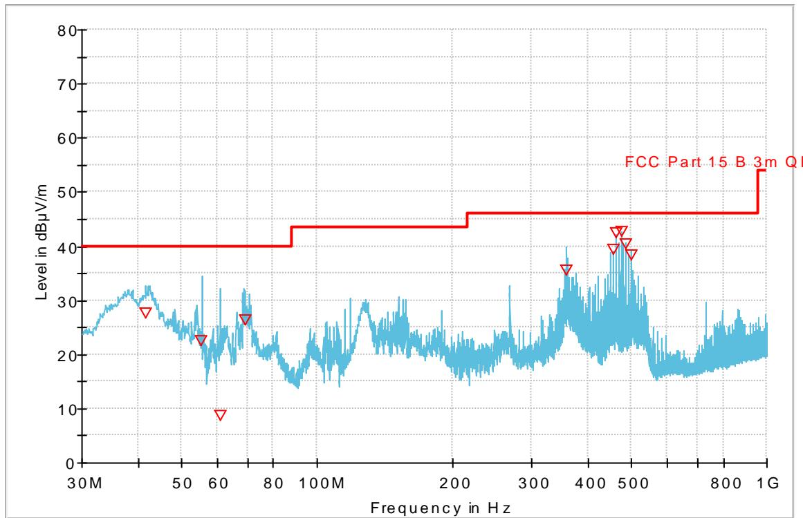
**Radiated Emissions, 30–1000 MHz, EUT V, Max VP/HP**
