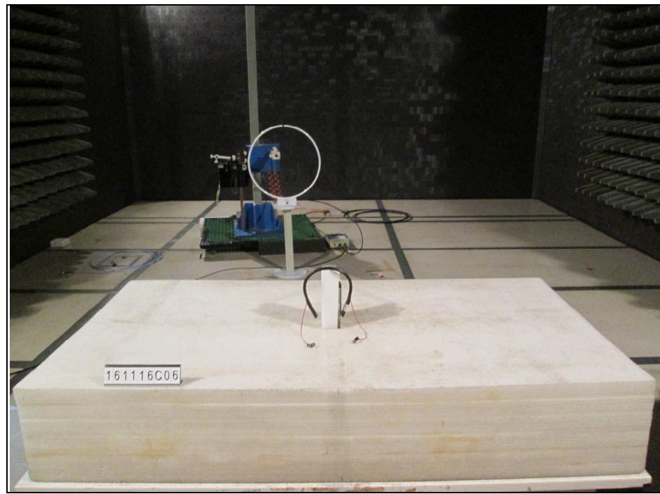
**For NFC: Radiated Emissions test (For frequency above 30MHz)**
