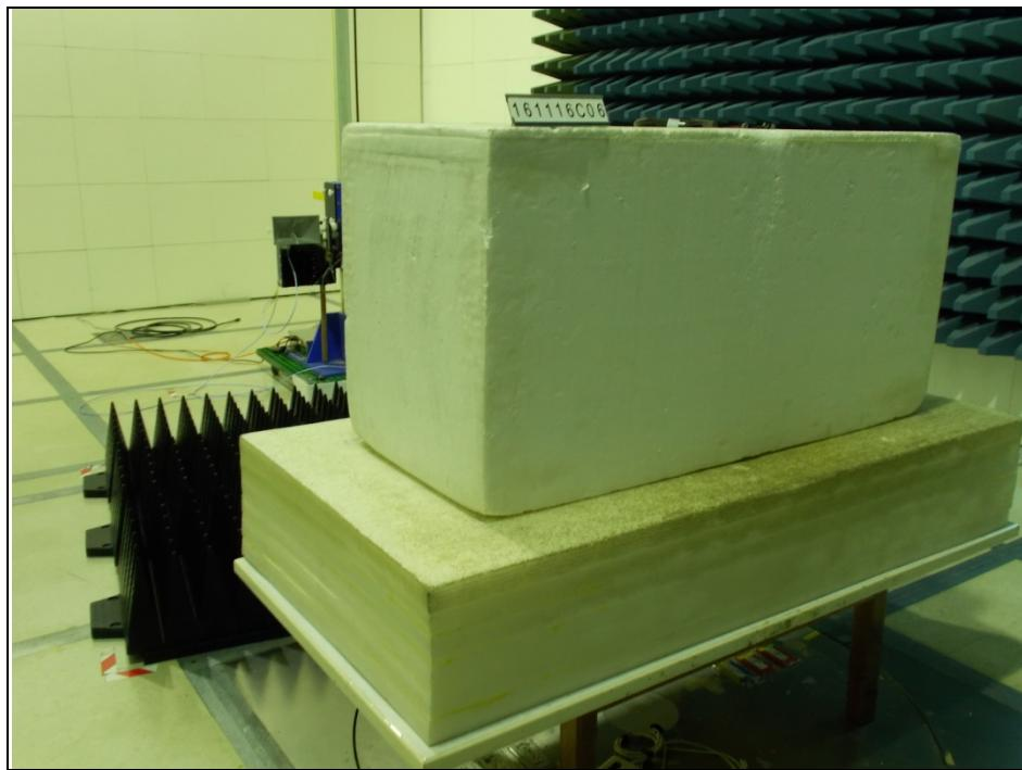
For NFC: Radiated Emissions test (For frequency range 9kHz ~ 30MHz)
