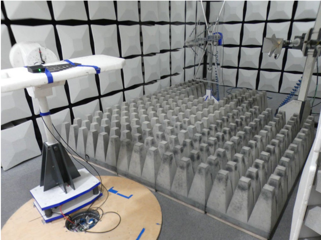
Photo 3: Setup Spurious Emissions Radiated (FAC), > 1GHz
