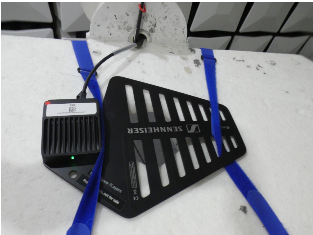
Photo 3: Setup Spurious Emissions Radiated (FAC), > 1GHz, detail view
