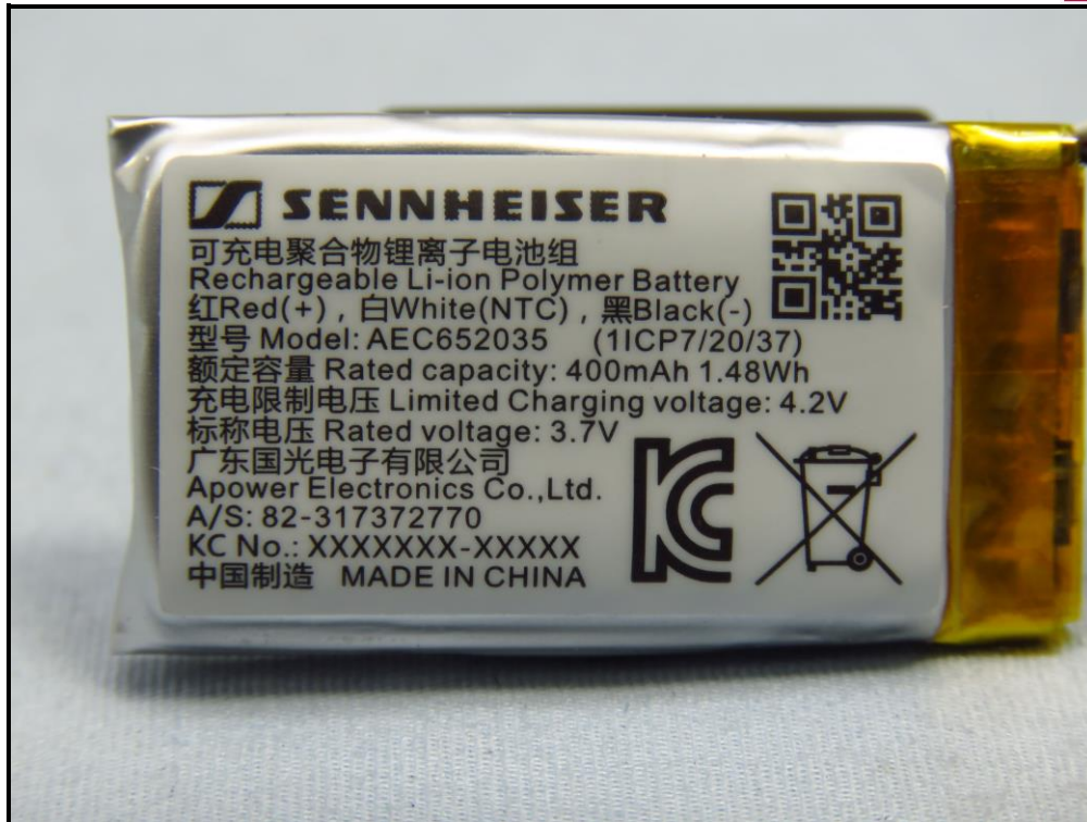
Earbud (alternative battery cell)
