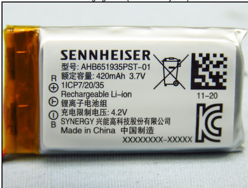
Charging case (Main battery cell)
