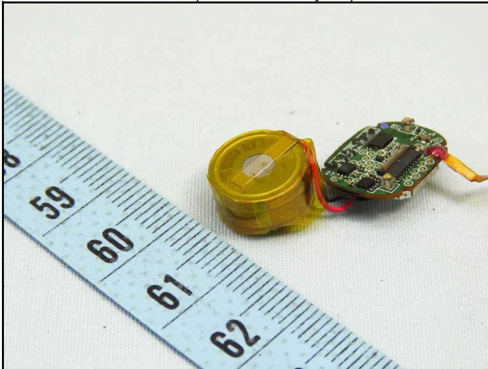
Earbud (alternative battery cell)
