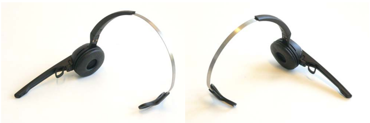
Fig. 13: Pictures of the D 10 HS with attached headband and rubber ear buds.
