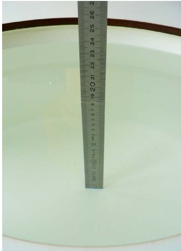
Fig. 16: Head liquid depth for 1900 MHz in flat part of the phantom.
