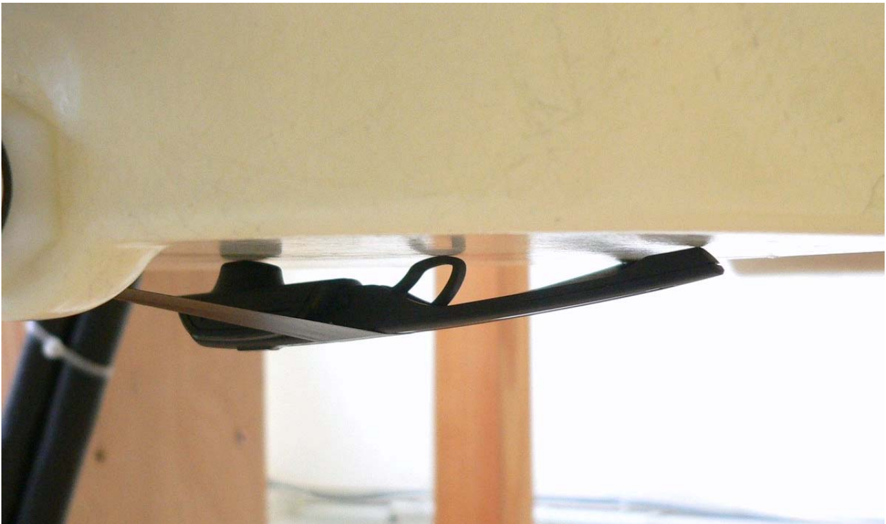
Fig. 14: Ear hook wearing style, test position 1 for the D 10 HS from Sennheiser Communications.
