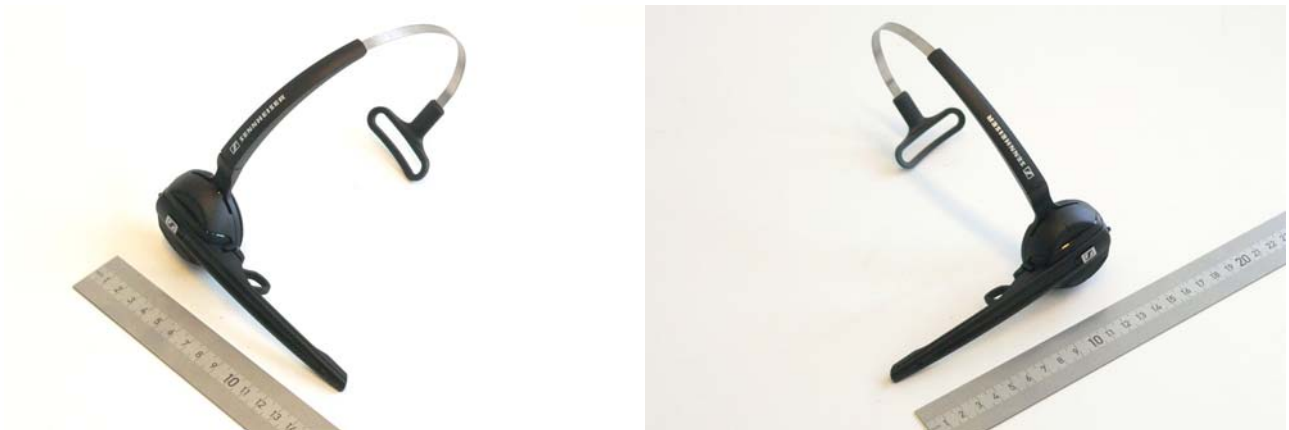
Fig. 12: Pictures of the D 10 HS under test with attached headband without rubber ear buds.
