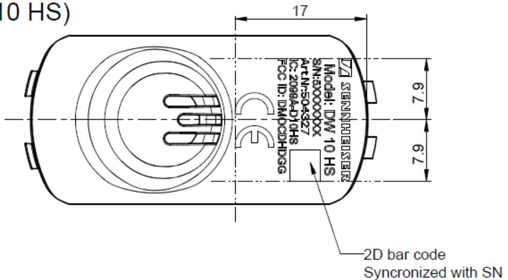
**Figure 1.1:** Label engraved on the surface of the DW 10 HS
