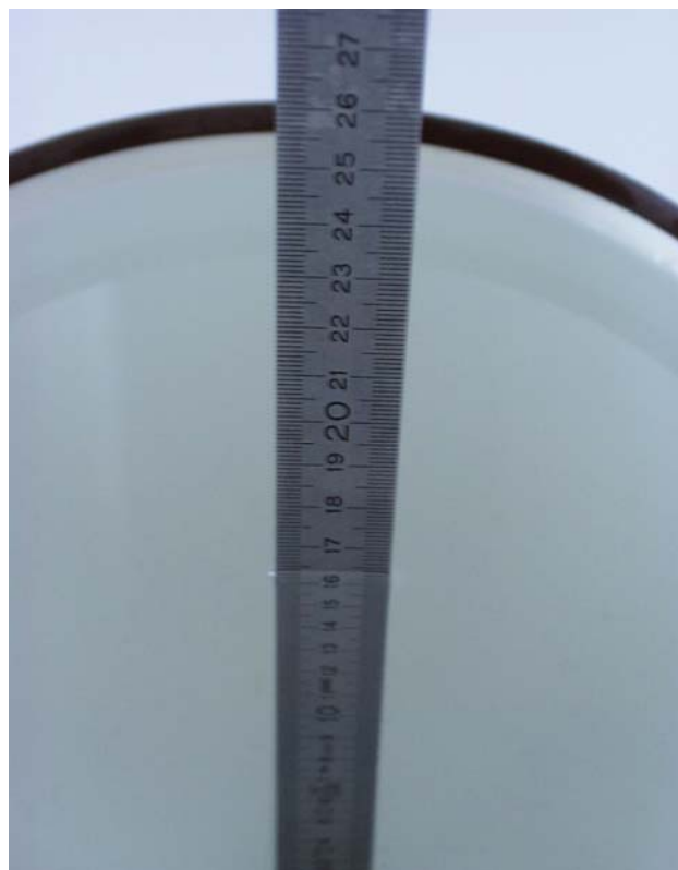
Fig. 15: Liquid depth for 1900 MHz Head measurements.
