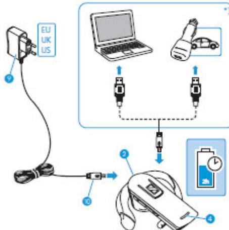
During charging, the LED ⑩ lights up blue. All ⑥ connections will be interrupted. When charging is complete, the LED goes off.
